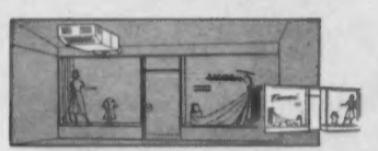
For stores, offices and other open areas, discharge return plenum eliminates need for cold air ducts.
